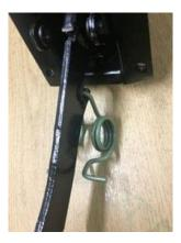
Rotate the spring around and use some good quality long nose mole grip or pliers to push the spring towards the bush.
